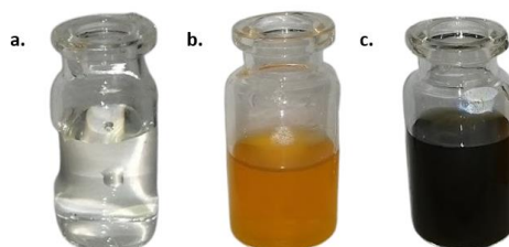
Figure 1. A visual transformation was observed during the green synthesis of iron nanoparticles (FeNPs-A) using aqueous avocado seed extract (Ext-A) as a reducing and stabilizing agent. a. Iron solution b. Avocado extract c. FeNPs-A
